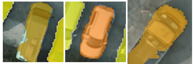
(a) Van misclassified as truck (b) Car misclassified as van (c) Pick up misclassified as van
