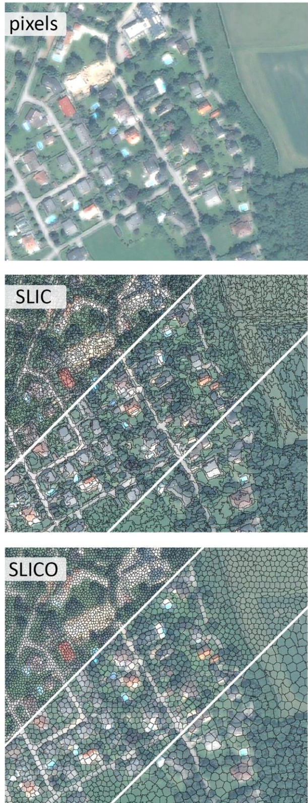
Figure 1. Visual comparison of superpixels produced by SLIC and SLICO methods, on a subset of T2. The average superpixel size in the upper left of the image is 5 \times 5 pixels, in the middle of the image is 10 \times 10 pixels and 15 \times 15 pixels in the lower right.
