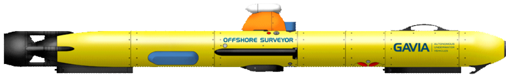
Figure 1: The Gavia Surveyor AUV showing typical modular payloads. From Right: nosecone, battery, DVL/INS (Kearfott T24), control with GPS and acoustic modem, GeoSwath, propulsion.
